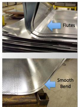
The photos to the left show sheets that were subjected to bending using a large radius. The bottom photo shows what is what is expected to occur when sheets are bent in a controlled manner – the curve is very smooth. When discontinuous yielding is present, the sheet will bend sharply every so often (flute) into a discontinuous curve that is totally unsatisfactory.
