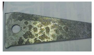
of zinc in the zinc hydroxide, zinc oxide, zinc carbonate sequence that happens over longer periods.
